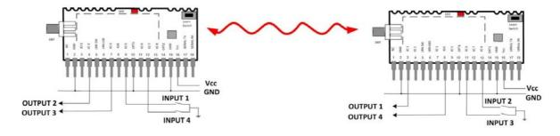
**NOTE:** GAMMA digital outputs are acitve high, but GAMMA digital inputs are active low. Therefore if connecting multiple GAMMA modules directly together, to extend range, the outputs will require inverting before applying to GAMMA inputs.
