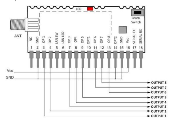
**Application Example:** Showing 4 transmitters paired to one single receiver - I/O used is arbitrary.
