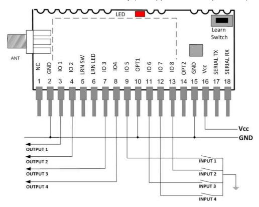
Application Example: Shows two GAMMA modules paired in both directions.
