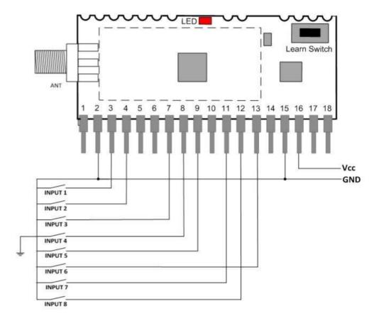
**Application Example:** Showing 1 transmitter paired to 3 receivers - I/O used is arbitrary.
